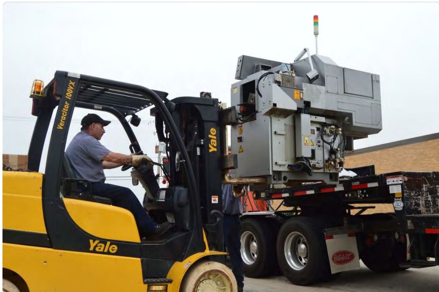
Workers remove via forklift the seven-axis Swiss CNC machines donated to Elgin Community College.
