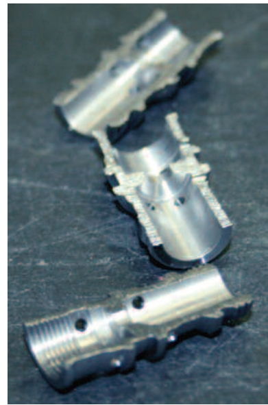
Some workpieces are bisected to ensure quality inside and out
